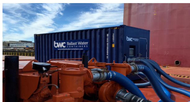
Fig. 2. Ballast water treatment in container designed specifically for the barge
